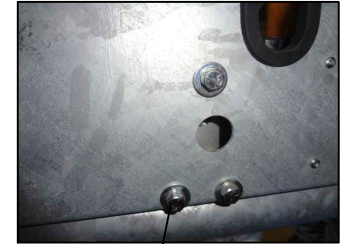
3 x \frac{5}{16} " bolt (2 \frac{1}{2} " long) (16) + lock washer (17)+ flat washer (23)
